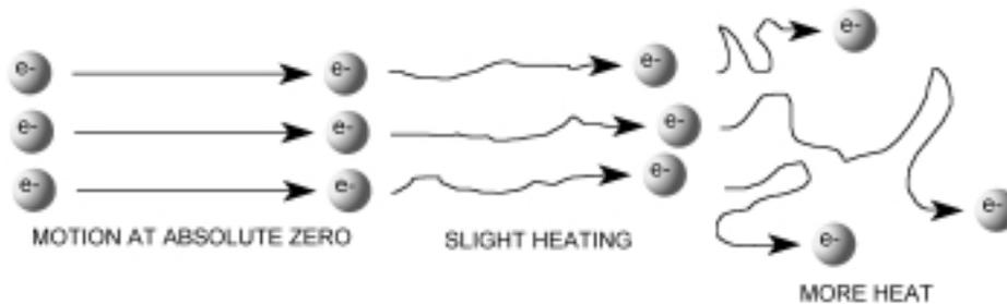
Figure 10-3. Thermal Noise
