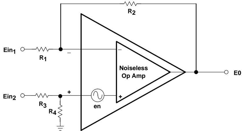
Figure 10–12. Differential Equivalent Op Amp Circuit Noise Model
