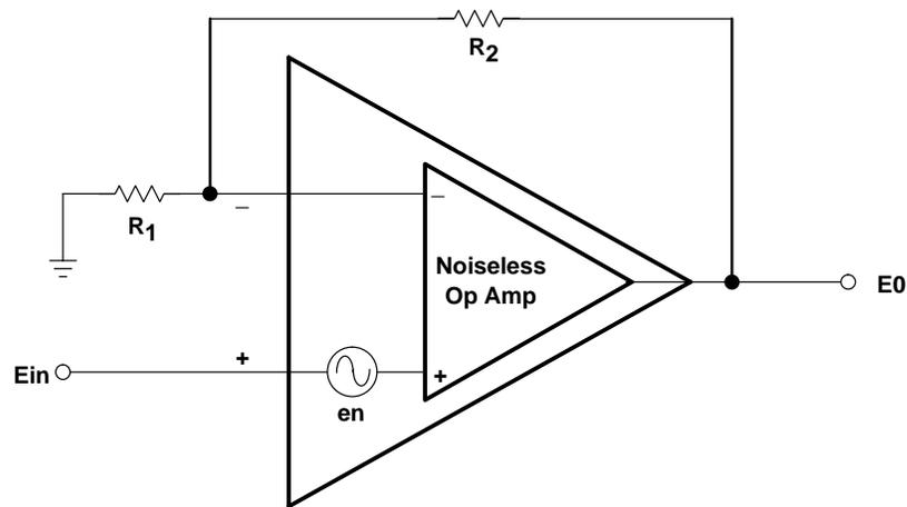
Figure 10-11. Noninverting Equivalent Op Amp Circuit Noise Model
