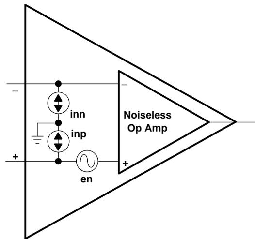
Figure 10–7. Op Amp Circuit Noise Model
